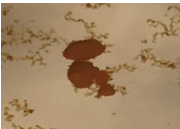
Pure curcumin sticking together on the surface of water and not dispersing
